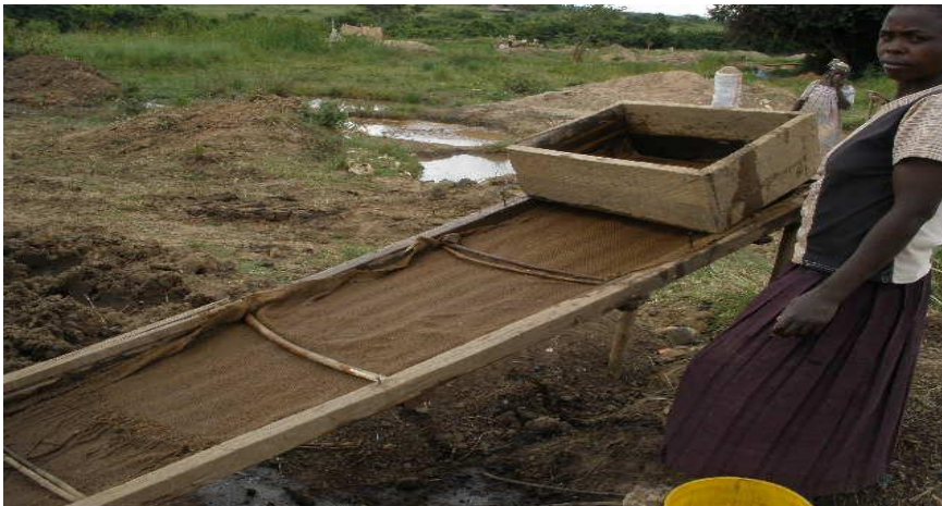
Plate 4.2: Gravity separation using a sluice bed. Process involves use of stream water hence allowing only the heavier materials to build up behind the riffles (Source: Author, 2007).
