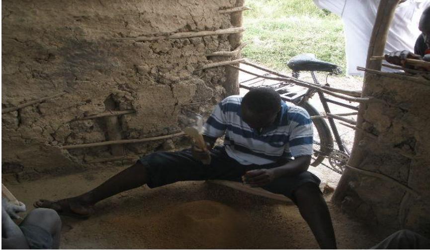
Plate 4.1: Fine grinding of gold ore (Source: Author, 2007).
